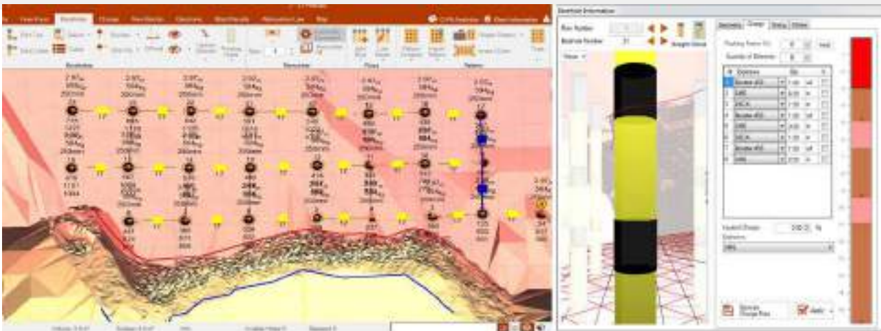
Fig 5: Blast design in O-PITBLAST
